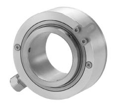
The ENC-C81 is a hollow shaft encoder used for heavy Industrial and Elevator feedback applications. These encoders are offered with resolutions ranging from 12 to 4096 CPR (model dependent). These encoders fit shaft diameters up to 44mm, but reducing sleeves are available for shaft diameters as small as 15mm. With various mounting options, three output circuitry options, and input voltage ranges, these encoders can be customized to fit your applications needs.
